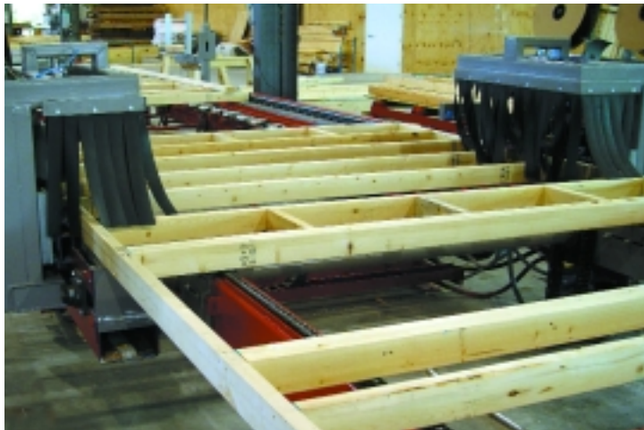
Sheathing and vapor barriers are pre-applied as needed during fabrication.
